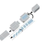
Stacking of the bags. The bags are tilted at the inlet of the pick and place cell. The bags are put into the boxes in horizontal position. The bags can be rotated in the horizontal plane, thanks to the rotation of the handling gripper.
